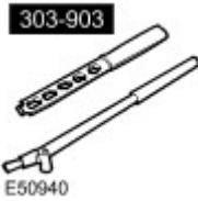
Oil seal remover 303-903 (LRT-12-092)
